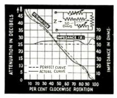
Fig. 4. Impedance and attenuation characteristics of a 50-ohm pad.
